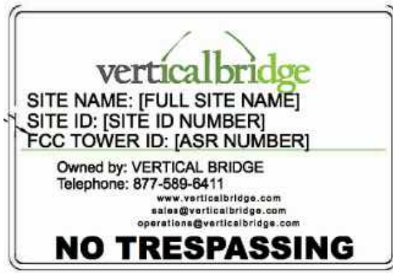
A | OWNER CONTACT SIGN 18" HIGH X 24" WIDE WHITE BACKGROUND, BLACK LETTERING MOUNTING LOCATION: LEFT GATE QUANTITY: 1
