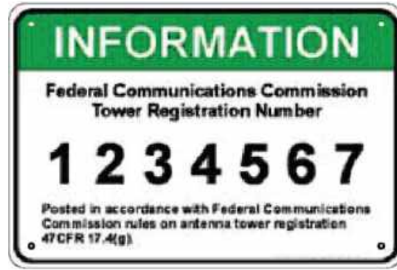
B | FCC REGISTRATION SIGN 8" HIGH X 12" WIDE WHITE/GREEN BACKGROUND, WHITE/BLACK LETTERING MOUNTING LOCATION: GATE & BASE OF TOWER QUANTITY: 2
