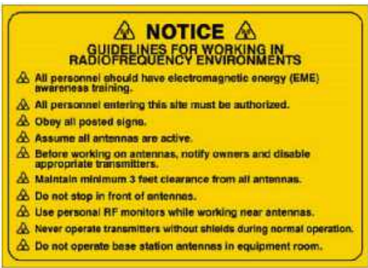
D | RF GUIDELINES SIGN 8" HIGH X 12" WIDE YELLOW BACKGROUND, BLACK LETTERING MOUNTING LOCATION: RIGHT GATE & BASE OF TOWER QUANTITY: 2
